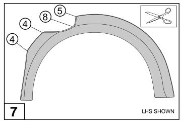
Cut a multiple triangles out of the extrusion where it meets the sharp corners as shown on the rear right flare. Note: Numbers of cut-outs indicated in circles.
