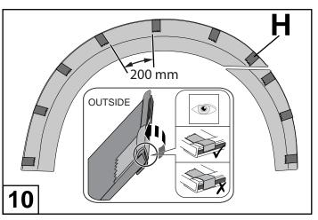
Apply masking tape as shown at 200mm intervals or where required to the fender flare extrusion. Fix the tape to the rear of the extrusion over the tape lining and over the front face of the Fender Flare. Ensure the tape does not overlap the tape lining and is not fixed to the inside surface of the fender flare.
