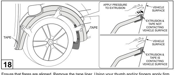
Ensure that flares are aligned. Remove the tape liner. Using your thumb and/or fingers apply firm pressure on the extrusion to ensure the extrusion and the tape is contacting the vehicle surface around the full perimeter of the flares.
