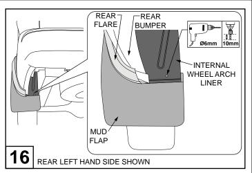
From the rear of the vehicle, clamp the Rear Mud Flap & (plastic) Internal Wheel Arch Liner. Using the hole in the Internal Wheel Arch Liner as a guide drill a Ø6mm hole through the Mud Flap as shown.
