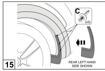
Fit the Mud Flaps to the Fender Flare and secure each Mud Flap with three (3) Scrivets supplied as shown.
