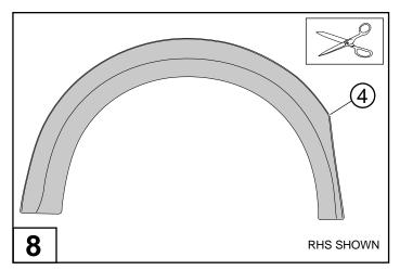
Cut a multiple triangles out of the extrusion where it meets the sharp corners as shown pn the rear left flare. Note: Numbers of cut-outs indicated in circles.
