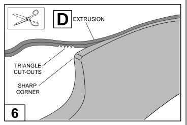
To fit the extrusion around sharp corners, cut a multiple triangles out of the extrusion where it meets the sharp corners as shown in steps 7 and 8.
