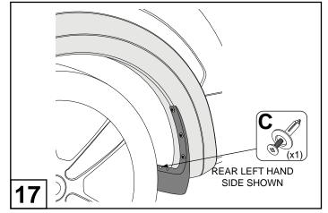
Fit one (1) Scrivet into previously drilled hole as shown.
