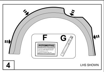
Clean the inside edge of each fender flare where the rubber extrusion will adhere with the Alcohol wipe and prime with the Primer Stick supplied.
